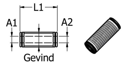
Ext. hose diameter A1 = 12 Ext. hose diameter A2 = 12 L1 = 40.7Thread = M20x1
